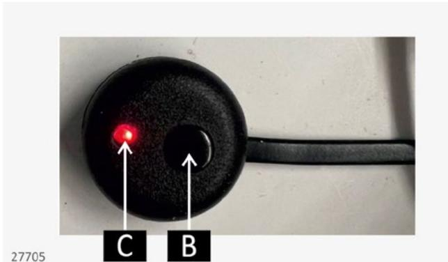
Press button [B] and check that the LED [C] flashes once every 30 seconds. In this condition, the interconnection system functions correctly.
