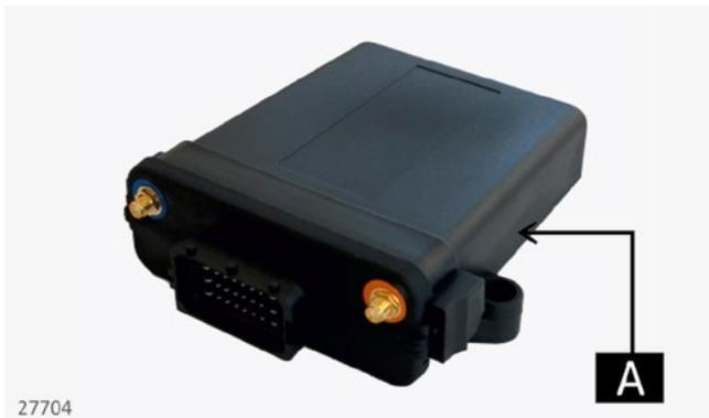
The operation of the system is based on the installation on Merlo machines of the MOVISAT SUPER NVT3 control unit, an IOT device capable of connecting with the machines' electronic systems in order to obtain telemetry and usage data.
